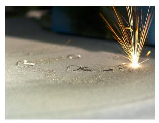
From security-related components to operating theatre equipment, the sheer range of 3D-printed parts is expanding by the day. This also increases the significance of Melt Pool Monitoring in guaranteeing their safe and cost-optimised production.
